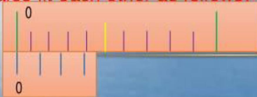
To take precise measurements, we have to ensure that the caliper we are using is of no zero error.
