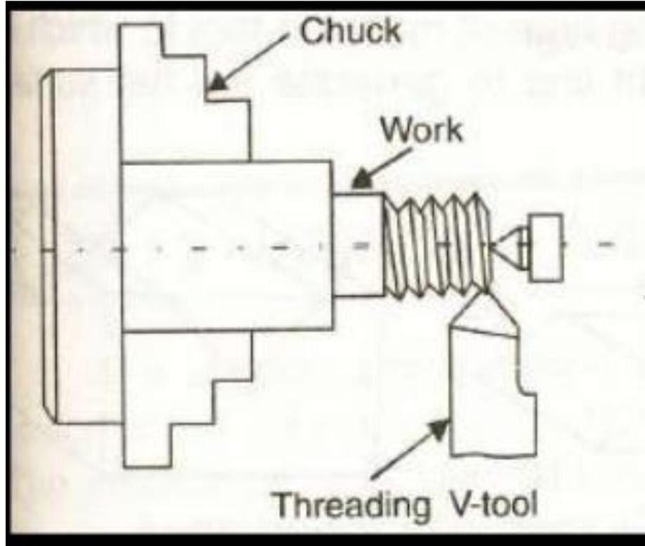
Threading is a turning operation in which a tool moves along the side of the workpiece, cutting threads in the outer surface. A thread is a uniform helical groove of specified length and pitch. Deeper threads need multiple passes of a tool.
