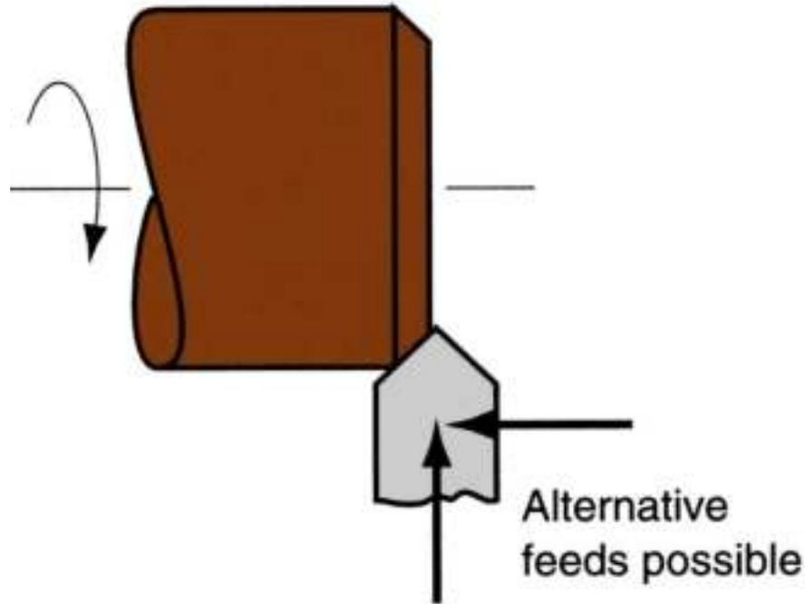
It is the operation of getting a bevelled surface at the edge of a cylindrical workpiece. This operation is done to remove burrs to protect the end of workpiece from being damaged and to have better look. This operation is done in case of bolt ends and shaft ends.
