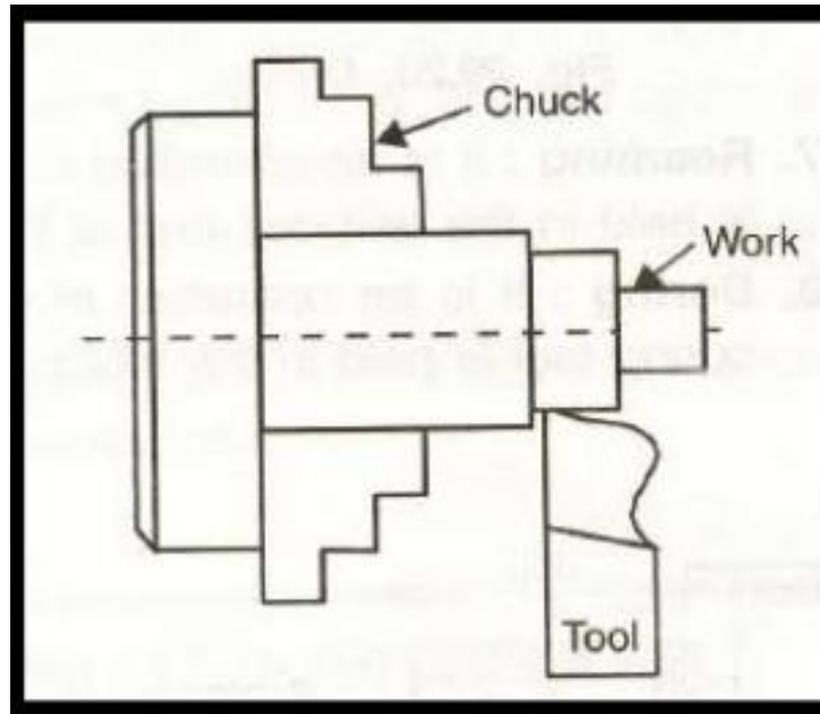
In stepped turning, the workpiece is turned in such a way that throughout the turning length it forms the steps of different diameters.
