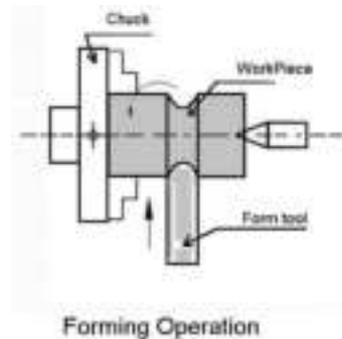
The centre of the tool is set slightly above the centre line of the work to provide an effective front clearance angle on the tool. The tool will rub against the work if the centres are of the same height.
