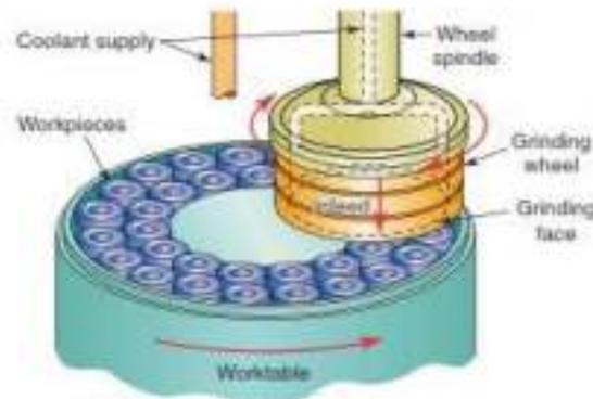
Figure L-5 Principle of the vertical spindle rotary grinder.
