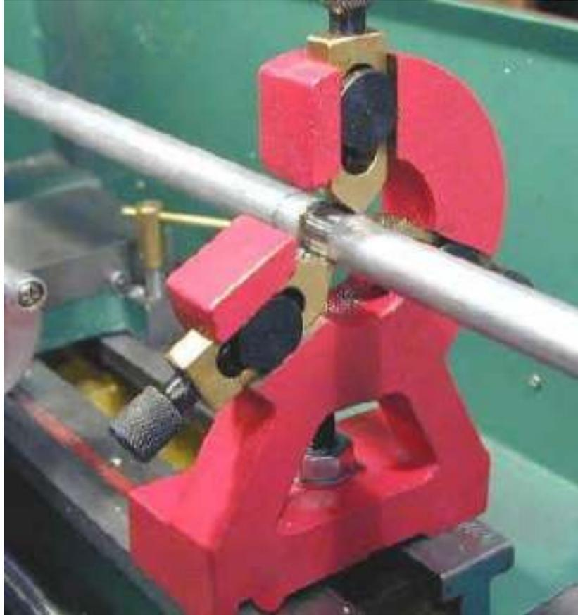
Steady rests are needed **when the length and stiffness of a workpiece makes it difficult to machine without distorting or deflecting the part.** This damage is the result of cutting or forming tool pressures that are simply too great for the part to withstand without additional support
