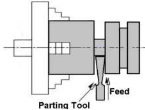
The width of the cutting edge range from 3 to 12 mm only. The length of the cutting tool which inserts into the work should be slightly longer than the radius of the bar stock being machined.
