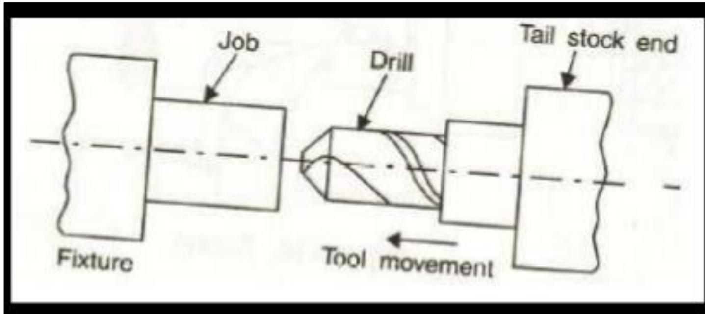
A drill enters the workpiece axially through the end and cuts a hole with a diameter equal to that of the tool
