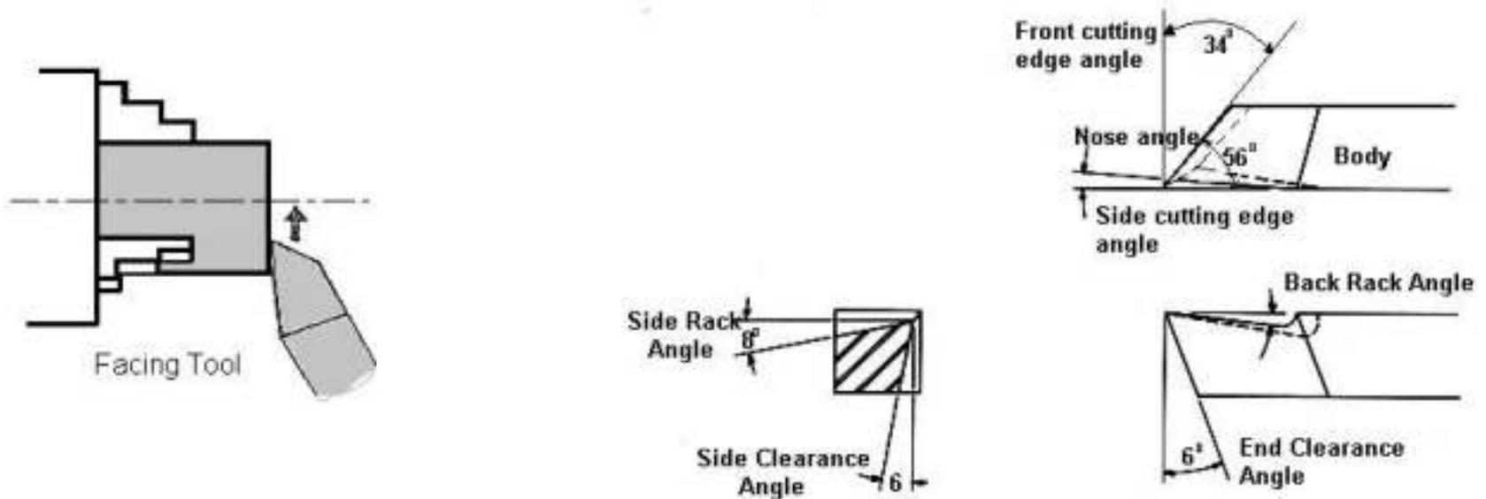
The tool has  $2^\circ$  side cutting edge angle and  $34^\circ$  end cutting edge angle can be accommodated in the space between the end of the work and  $60^\circ$  dead centre leaving a clearance of  $2^\circ$  on both sides.
