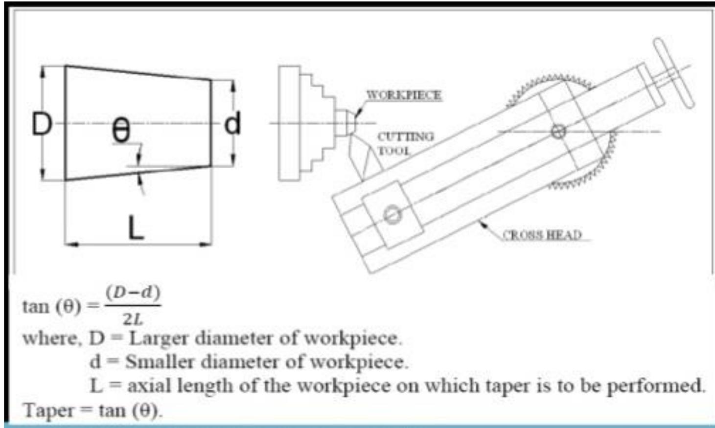
A "taper" is the uniform increase or decrease in the diameter of the workpiece and measured along with its length.
