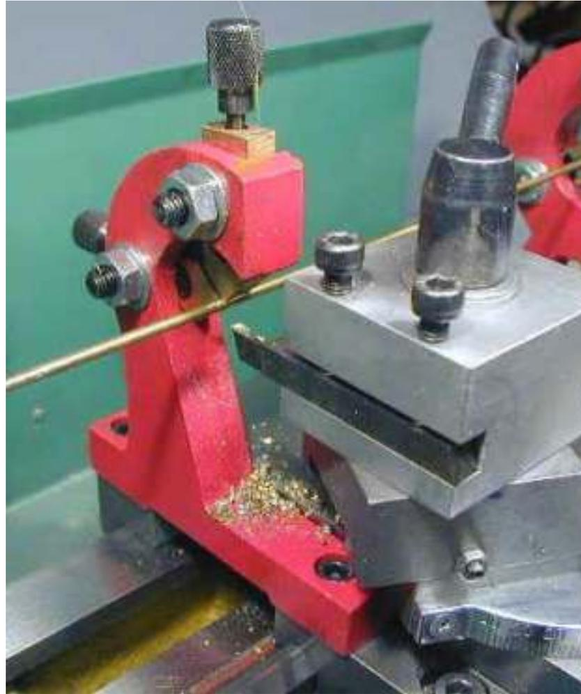
The purpose of the follower rest is **to keep long or small diameter work from deflecting when a cutting tool is applied to it.** It is attached to the lathe saddle and moves as the saddle moves, keeping the point of support directly behind the cutting tool.
