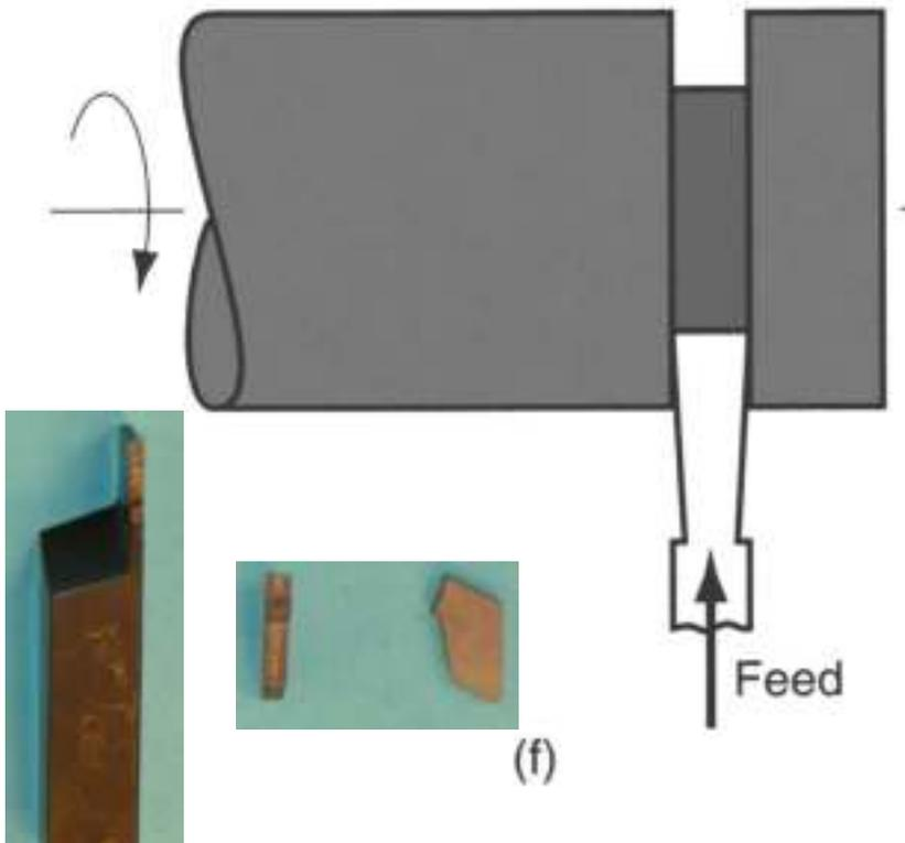
Tool is fed radially into rotating work at some location to cut off end of part, or provide a groove
