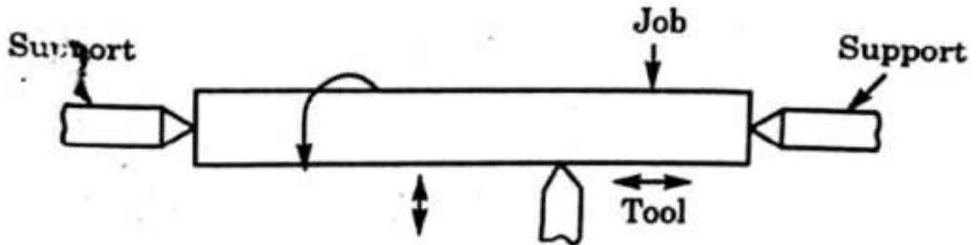
**Working Principle:** The lathe is a machine tool which holds the workpiece between two rigid and strong supports called centers or in a chuck or face plate which revolves. The cutting tool is rigidly held and supported in a tool post which is fed against the revolving work
