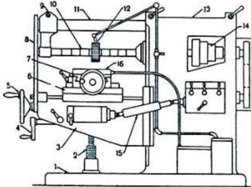
1. Base, 2. Elevating screw, 3. Knee, 4. Knee elevating handle, 5. Crossfeed handle, 6. Saddle, 7. Table, 8. Front base, 9. Arbor support, 10. Arbor, 11. Overhanging arm, 12. Cutter, 13. Column, 14. Cone pulley, 15. Telescopic feed shaft.
