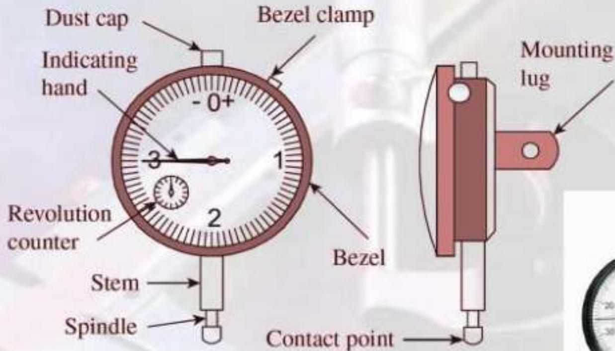
**Fig. 6.2** Functional parts of a dial indicator
