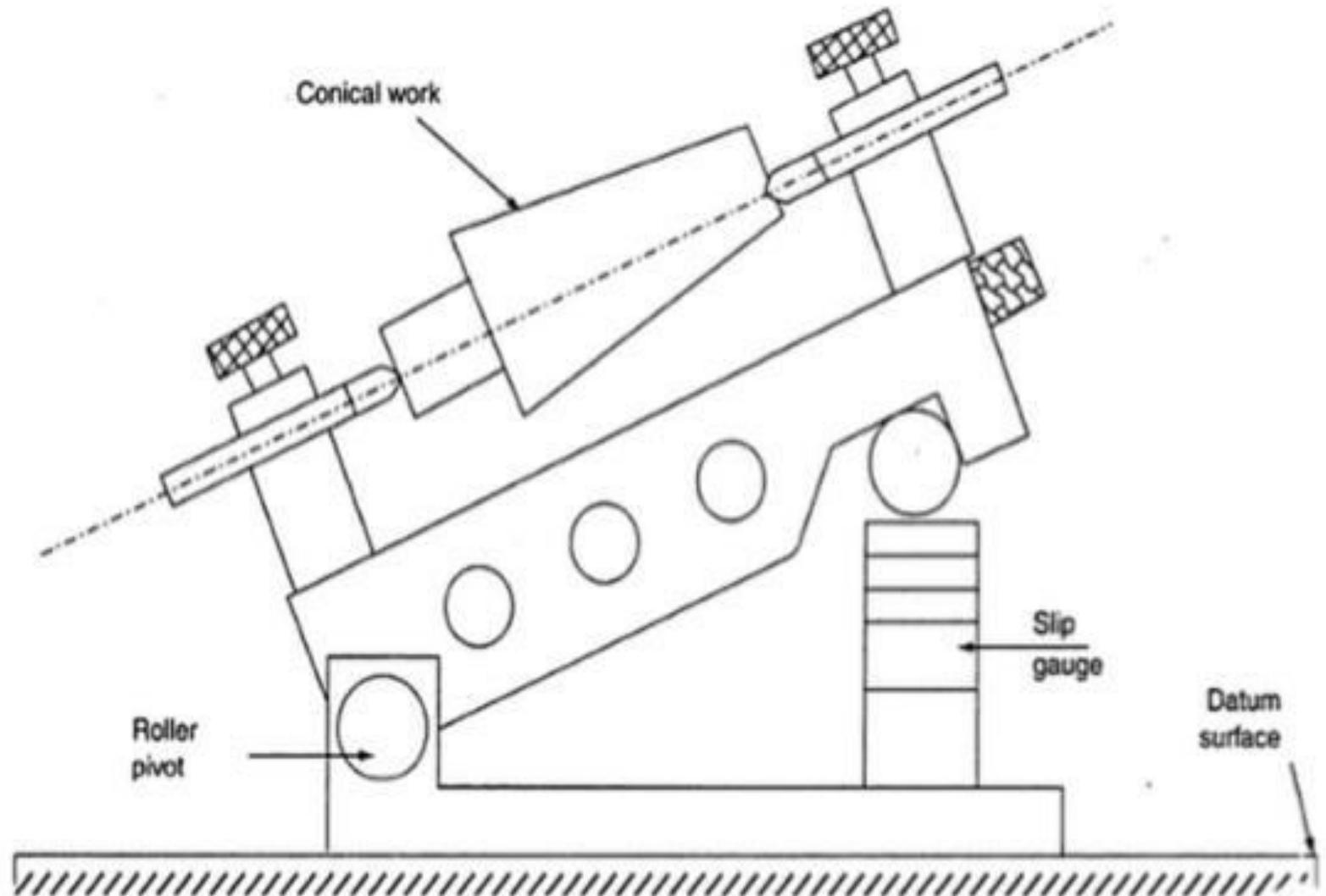
Measurement of included angle of taper plug gauge using sine cer\*
