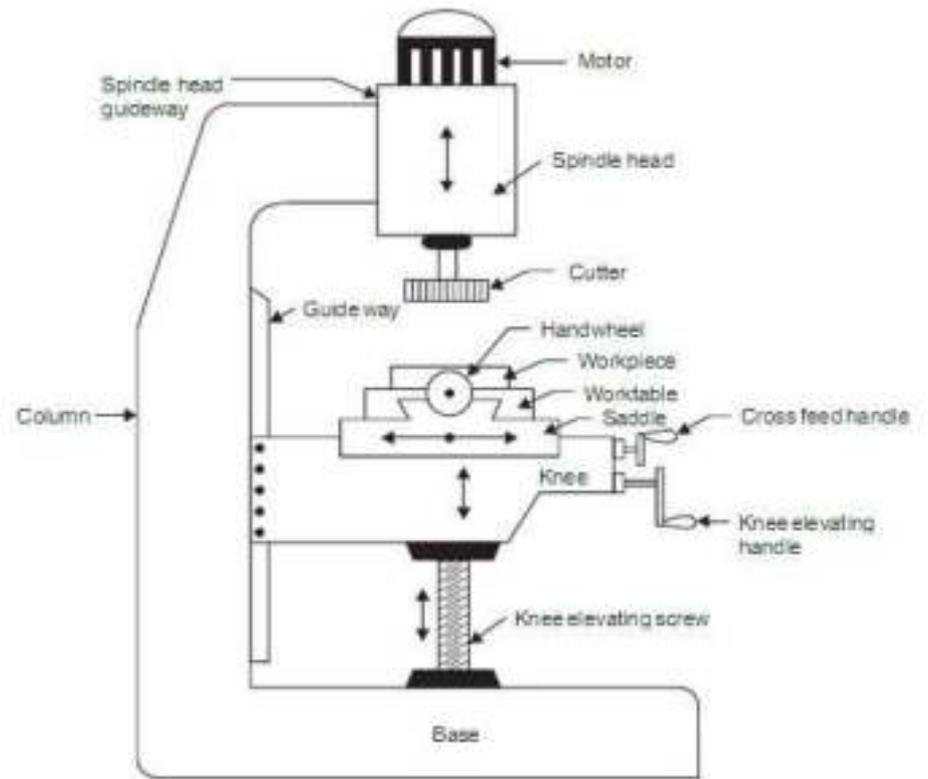
Fig. 4.10 Vertical milling machine
