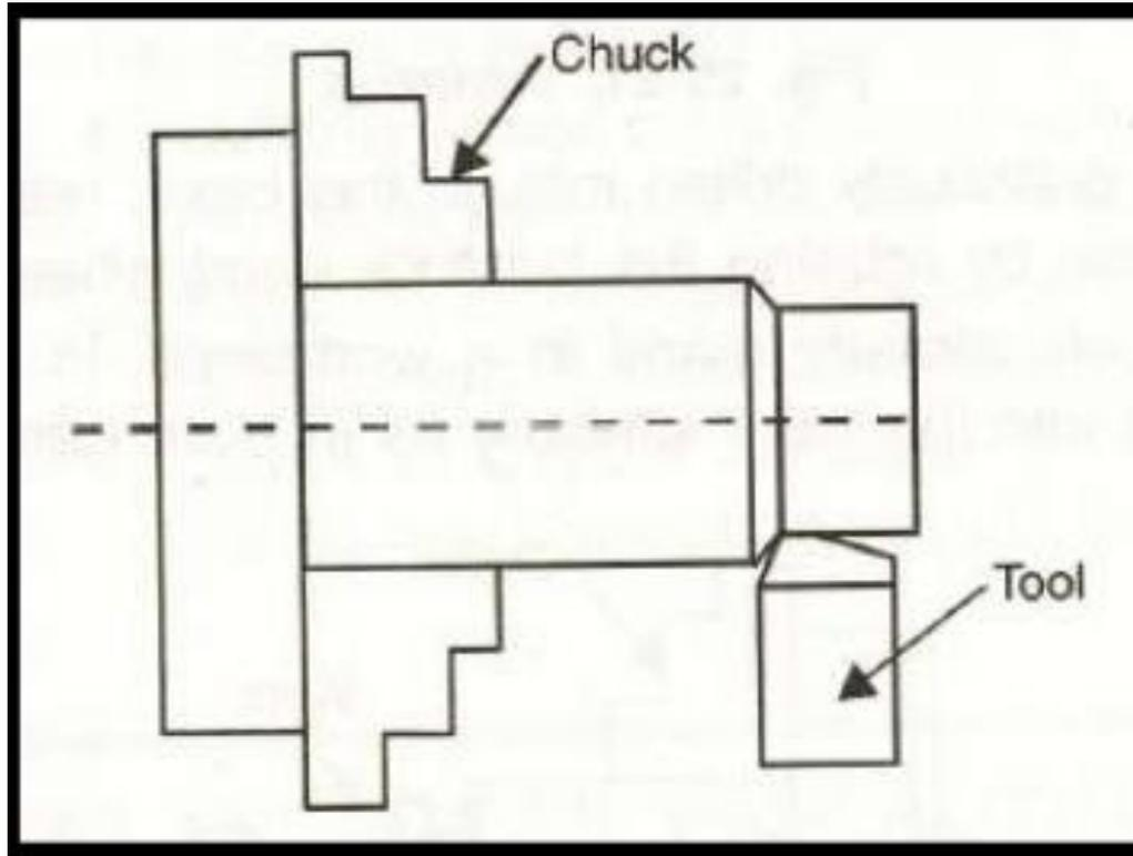
A single-point turning tool moves axially, along the side of the workpiece, removing material until the end diameter is reached.
