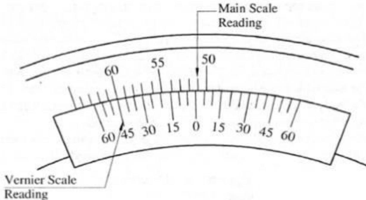
Thus the reading of the vernier bevel protractor equals :
