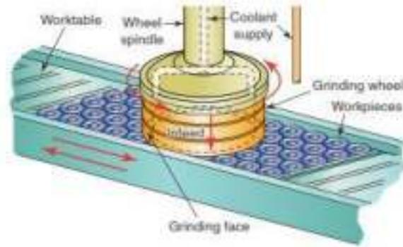
Figure L-4 Principle of the type II surface grinder, which has a vertical spindle and a reciprocating table.
