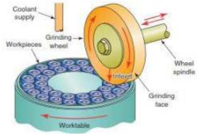
Figure L-3 Principle of the type II surface grinder. Sometimes circular parts are centered on this grinder; the resulting concentric scratch pattern is excellent for metal-to-metal seals of mating parts.
