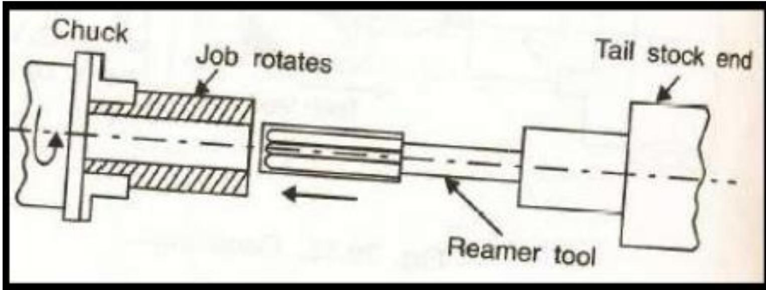
Reaming is a sizing operation that enlarges the hole in the workpiece. In reaming operations, reamer enters the workpiece axially through the end and expands an existing hole to the diameter of the tool. Reaming removes a minimal amount of material and is often performed after drilling to obtain both a more accurate diameter and a smoother internal finish.
