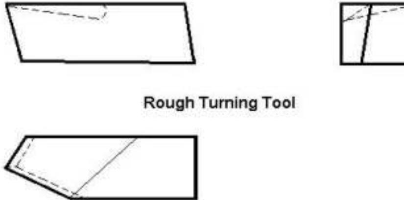
The main function of a rough turning tool is to remove the maximum amount of metal in minimum time that the tool, work, and the machine will permit. The cutting angle is so ground that it can withstand maximum cutting pressure.
