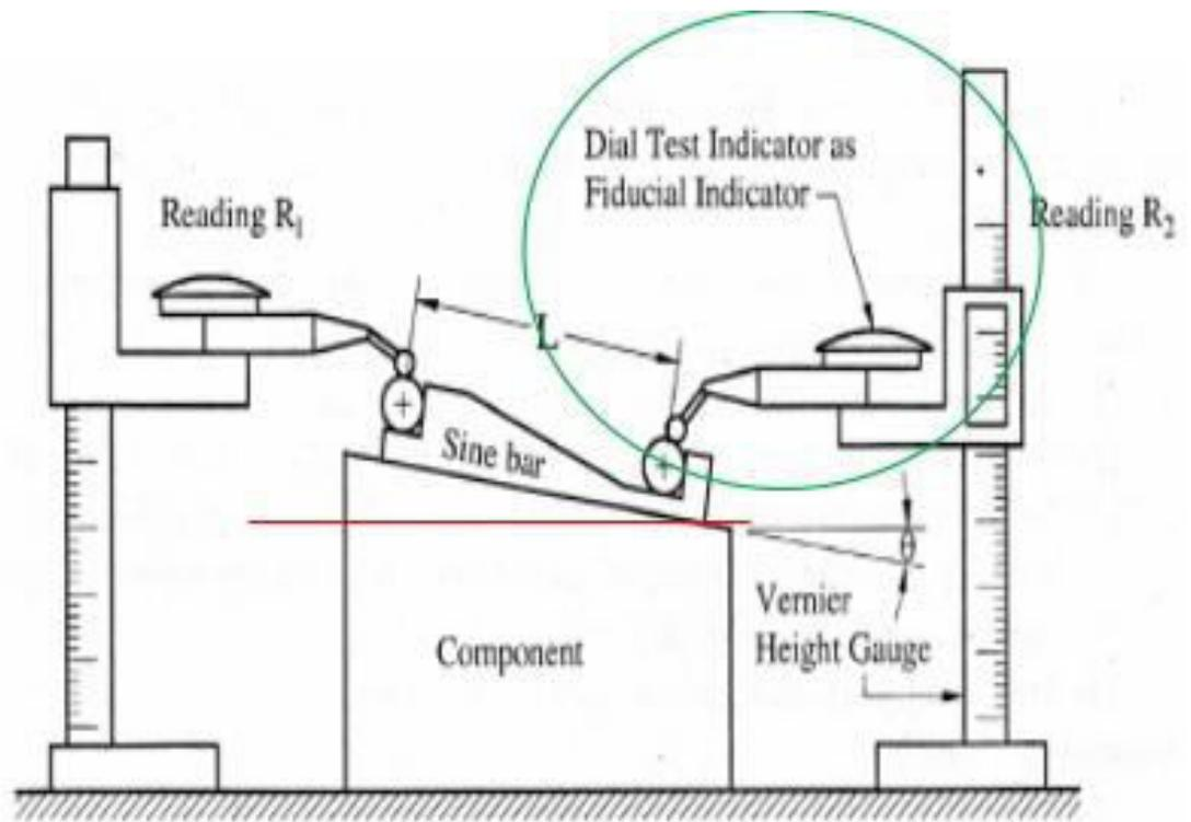
Fig. 3.10 Measuring angle of large size component.
