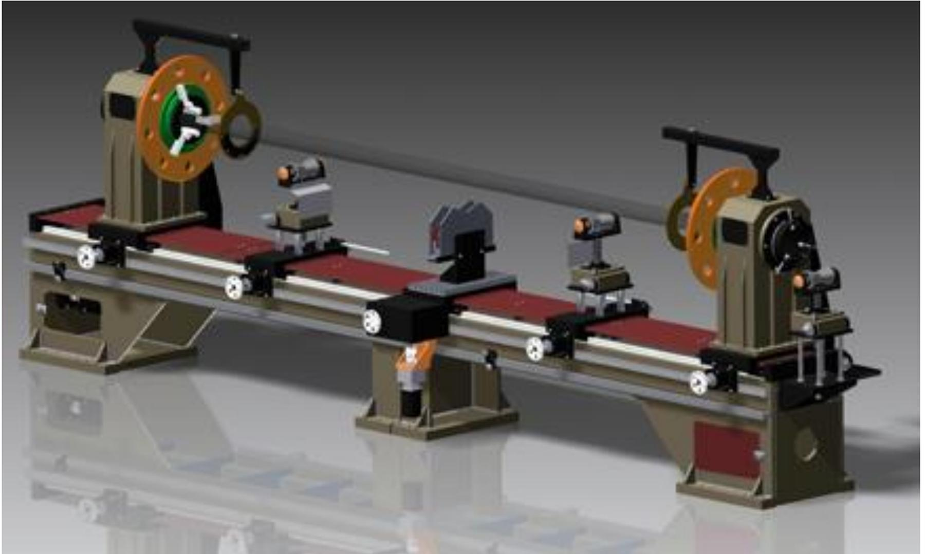
**Automatic lathe** - high speed, heavy duty, mass production lathe. Once tool is set, machining is done automatically, to obtain finished product.
