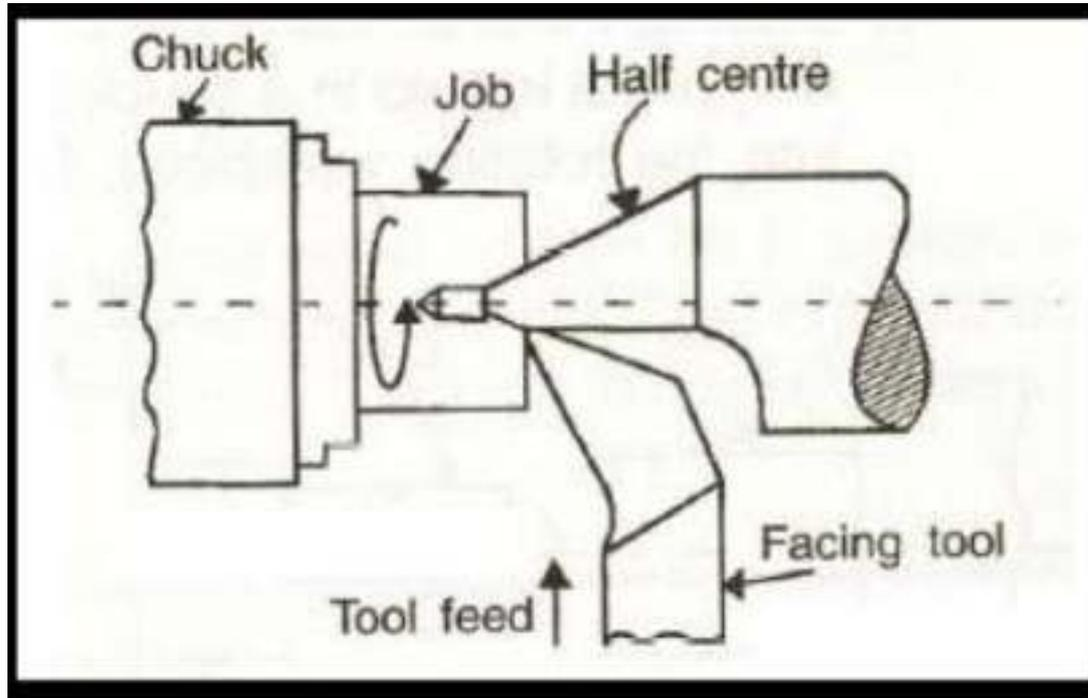
It is the machining of the ends of a workpiece to make the ends smooth. For this operation, the cutting tool is fed perpendicular to the lathe or workpiece axis by means of cross slide
