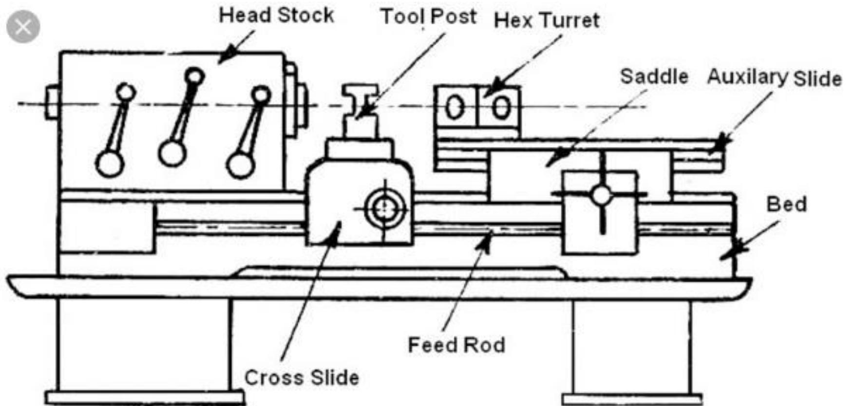
**Special purpose lathe** - used for special purpose and for jobs which cannot be machined on a standard lathe.
