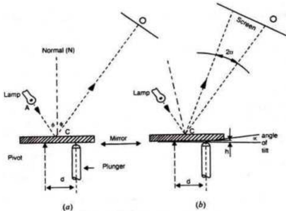
Fig. 1.14. Principle of the optical lever.
