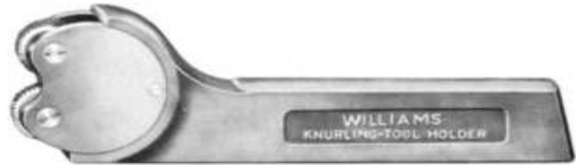
Knurling tool with one pair of rolls
