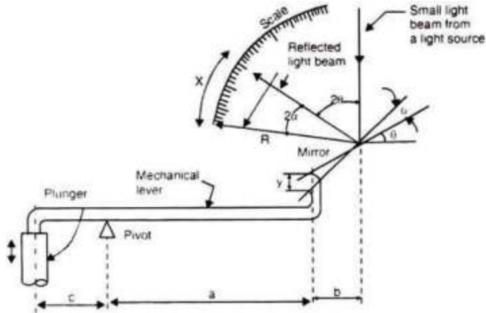
Fig. 1.15. An Optical Comparator.
