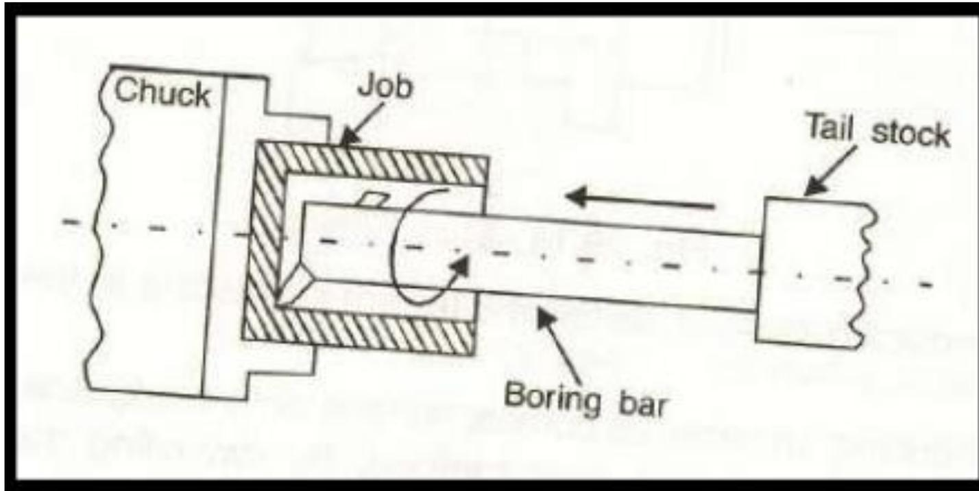
Boring process is performed to enlarge initial hole made by drilling process or to convert cylindrical hole to a taper hole.
