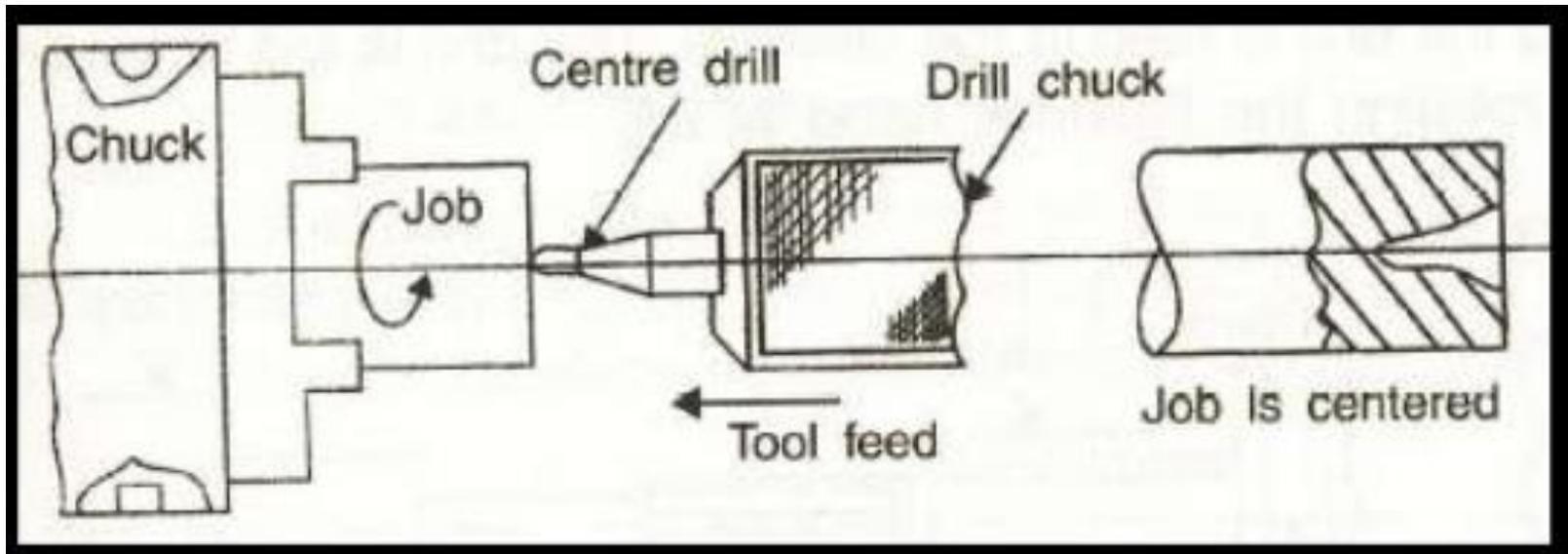
Centering is the operation of producing conical holes in the workpieces.
