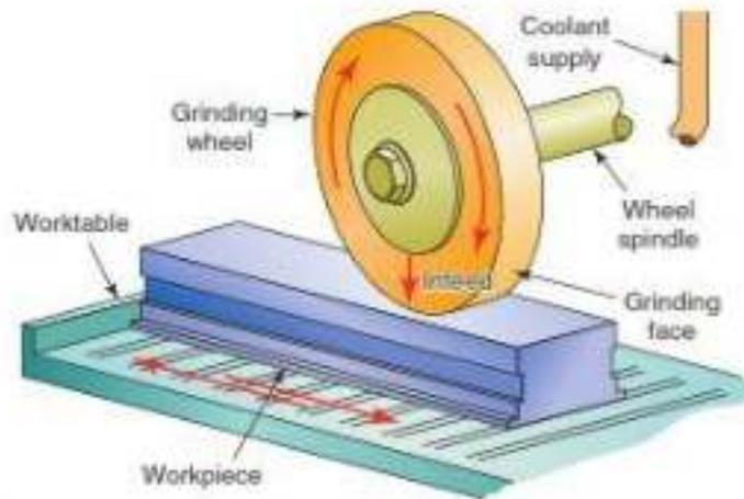
Figure L-1 Principle of the type I surface grinder.
