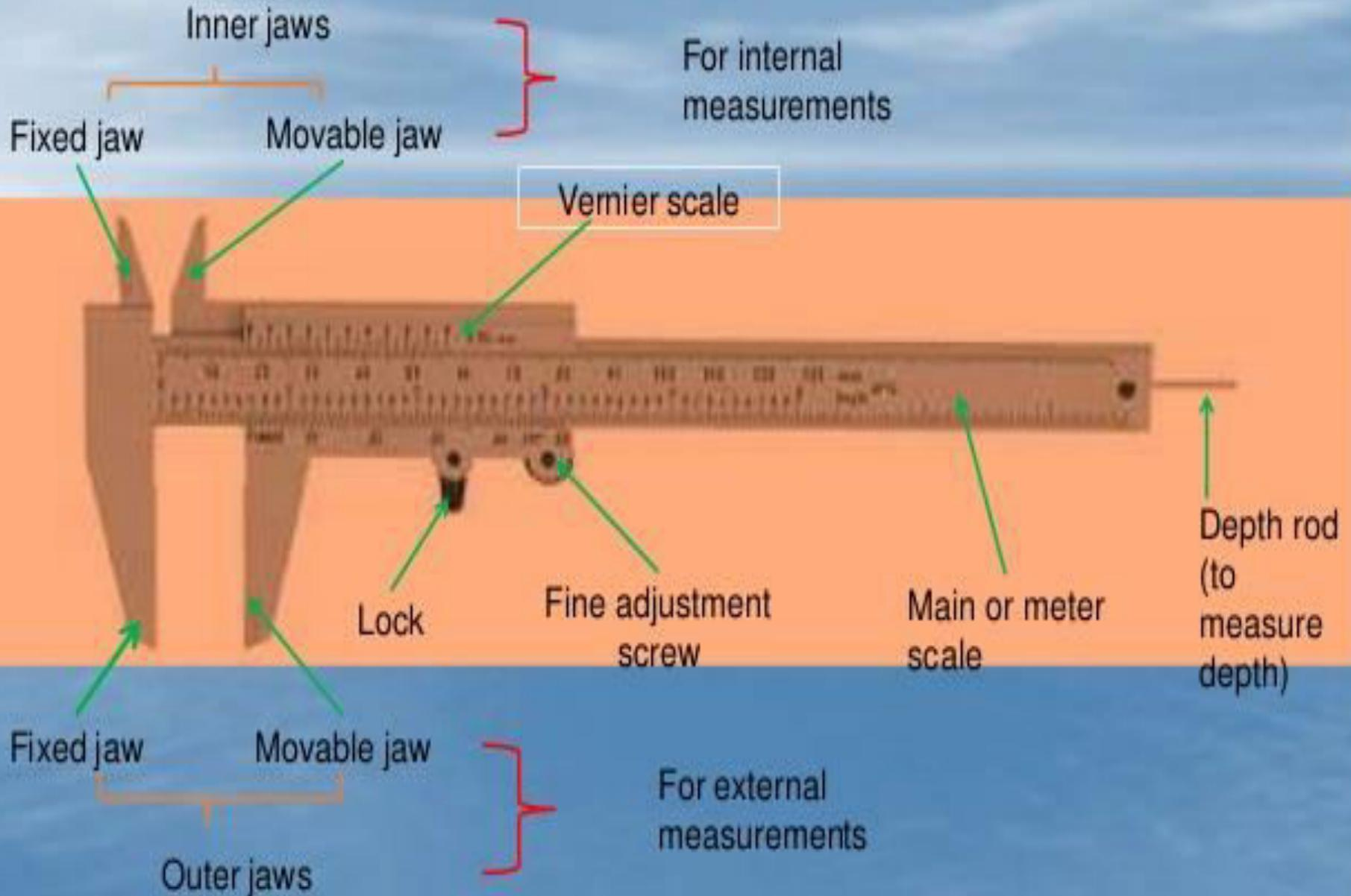
**1.Main Scale** - The main scale is similar to that on a ruler, graduated in mm and cm on one side ; inches on the other side.
