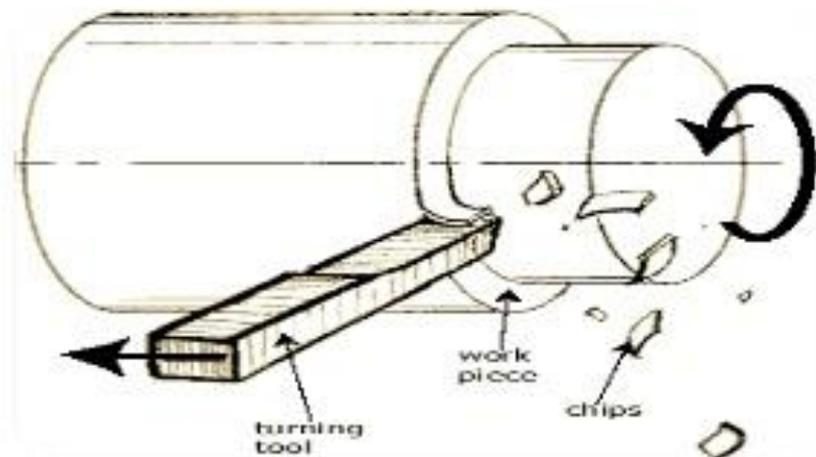
Turning is the removal of metal from the outer diameter of a rotating cylindrical work piece. Turning is used to reduce the diameter of the work piece, usually to a specified dimension, and to produce a smooth finish on the metal. Often the work piece will be turned so that adjacent sections have different diameters.
